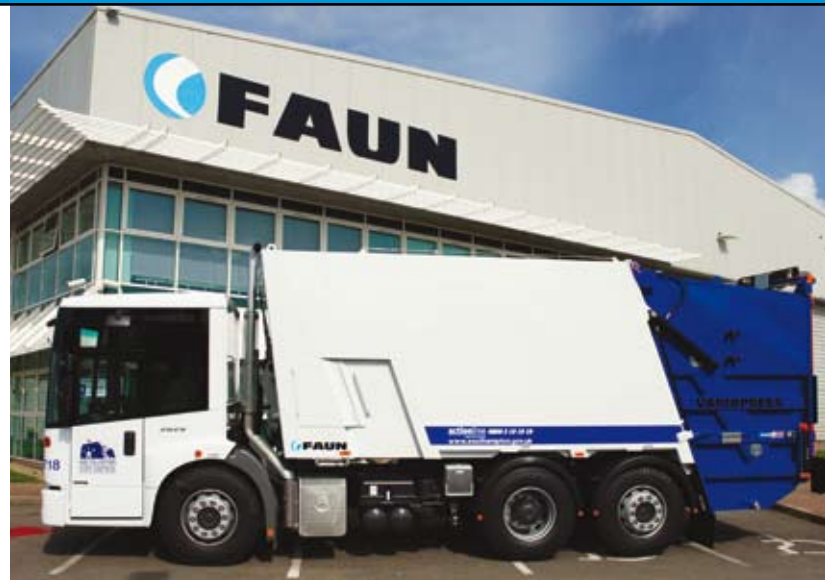
FAUN VARIOPRESS 20 cu m body mounted on Eonic 6 x 2 rear steer, 26 tonne chassis.
