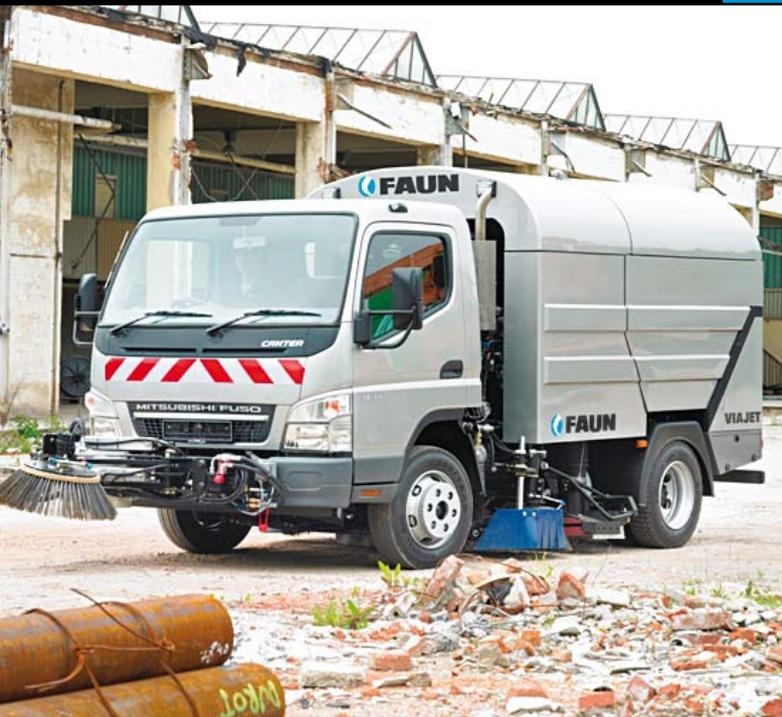
FAUN, Grimma Germany has brought its sweeper innovation to the smallest FAUN sweeper in the VIAJET range. The 4 cu m body is small, nimble and powerful. It has a choice of sweeping concepts, the FAUN air circulation system or mechanical sweeping unit.
