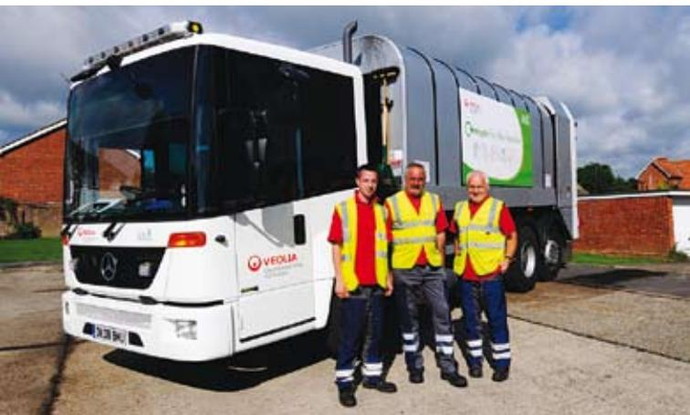
*Veolia ROTOPRESS 21 cu m body mounted onto Mercedes Eonic 26t rear steer chassis with automatic split lifter working on the West Berkshire contract*
